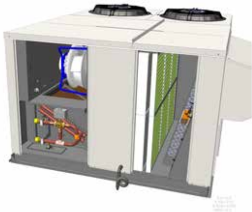
Figure 17 - Hot water coil location in the unit
