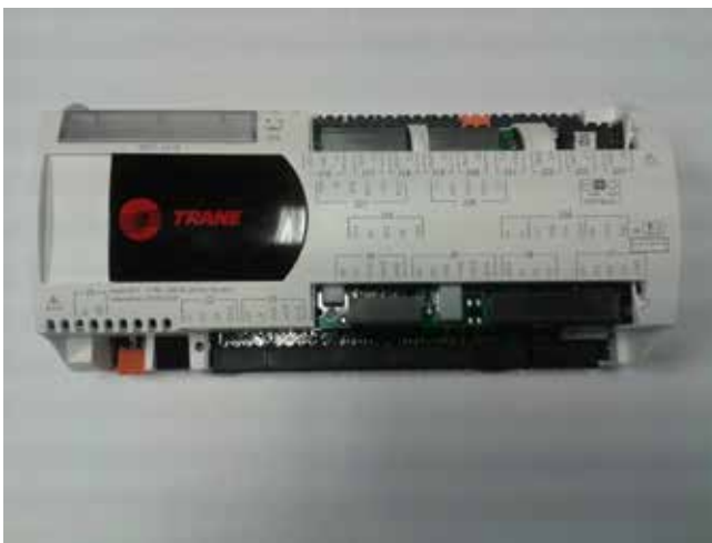
Figure 37 - CH536 main module
